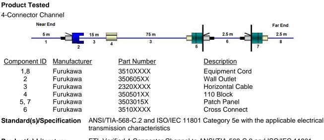
Product(s) Literature May Include: ETL Verified 4-Connector Channel to ANSI/TIA-568-C.2 and ISO/IEC 11801 Category 5e, along with channel illustration, and parts numbers.
