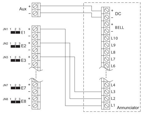
Connect panel's "+ AUX" contact to annunciator's "+ DC" contact. Connect panel's "- AUX" contact to annunciator's "- DC" contact. Connect panel's "+ E1" contact to annunciator's "L1" contact ...and so on.
