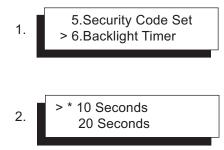
Press the "Down" switch to move to item 6 Backlight Timer. Press "Enter" switch to open the Backlight Timer.
