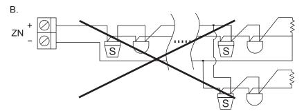
Wiring Diagram B. Improperly connected. Do not connect a detector or a end of line resistor in parallel with another detector.
