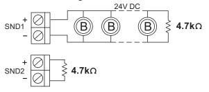
Fire alarm control panel is equipped with two set of Area Bells contacts. When connecting one set of bell contacts, be sure to connect the end of line resistor to avoid bell malfunction.
