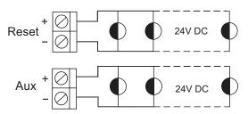
The contacts marked "24V" are controlled by the reset switch but the contacts marked "AUX" are not. When connecting the indicating lamp to the contacts, connect the red wire to the "+" and the black wire to the "-" contact.
