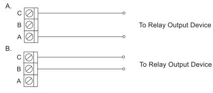
In picture A shows N.O. connection In picture B shows N.C. connection. (6) Fire/Fault Relay Output to Each Zone (Option) :
