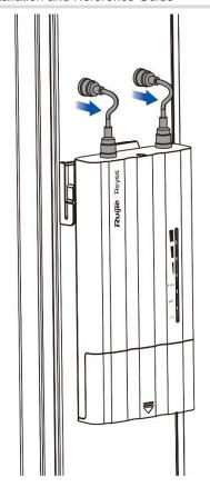
(3) Remove the wireless bridge by pulling it upward and then outward.
